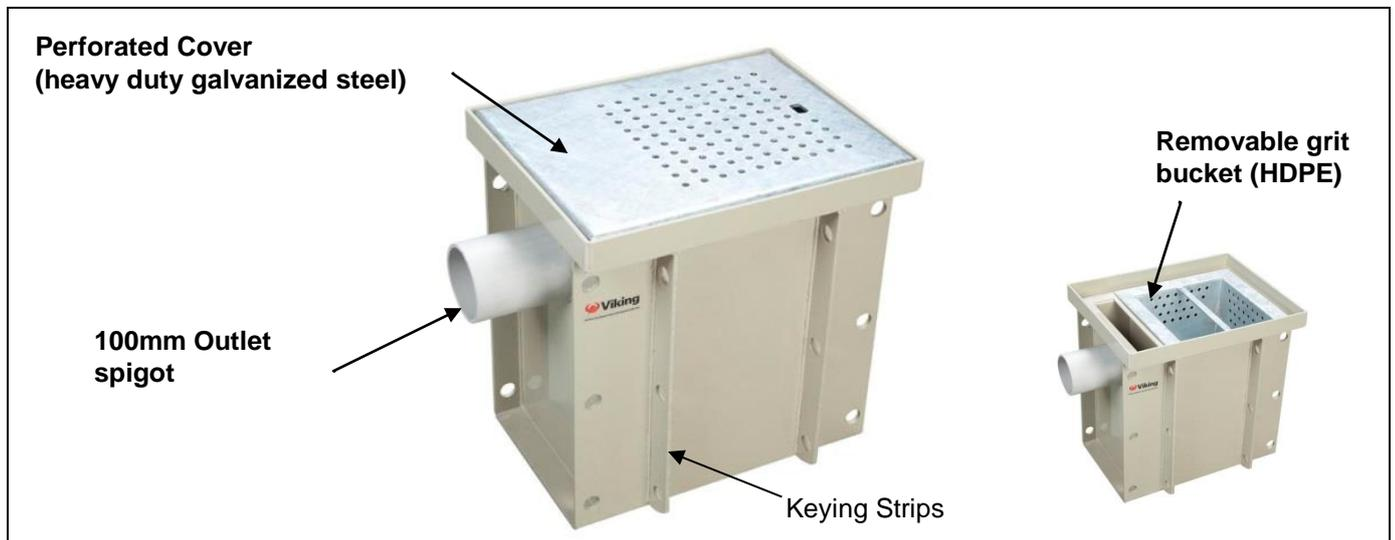
The silt pit is designed to be installed in a car or truck wash down bay. The top of the lid is at surface level. The lid is easily removed to gain access to the grit collection bucket fitted to the pit. The pit is to be surrounded with at least 100mm of concrete.
