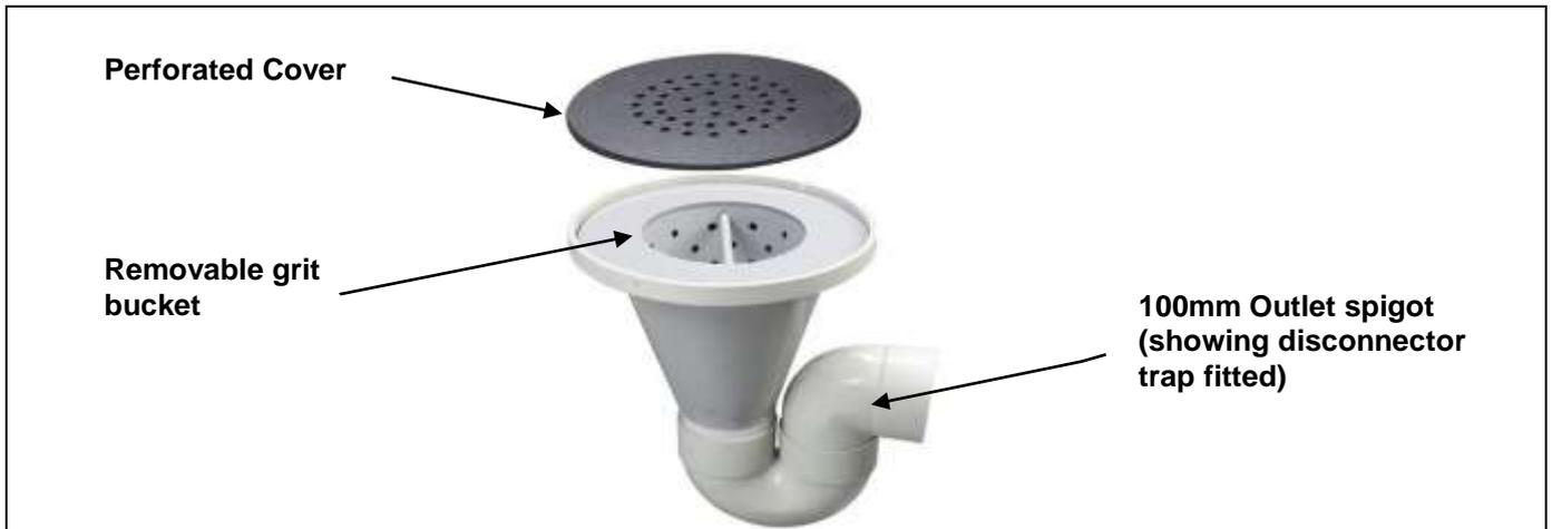
The silt trap is usually installed in a kitchen floor or an area where frequent wash downs are required. The top of the lid is at floor level. The silt trap is usually supplied with a 'disconnector trap'. The lid is easily removed to gain access to the grit collection bucket fitted to the trap. The body of the trap is to be surrounded with at least 100mm of concrete.
